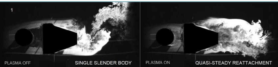
Visualization of flow around a landing gear-like configuration showing the ability of plasma actuation to stabilize the wake
